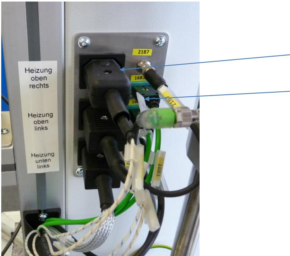
3x Heating sensor socket
